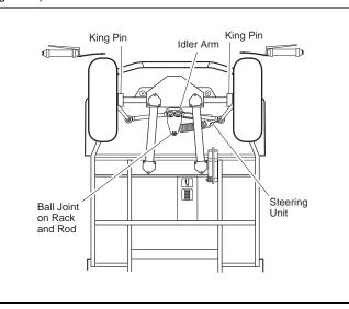
Fig. 29 Lubrication Points
